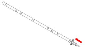
1. Insert the steel rod end of the male Shaft into a Bevel Gear. Push the Bevel Gear until it reaches the end of the platform (Make sure to match "D" shape of Bevel Gear hole to that of the shaft).
